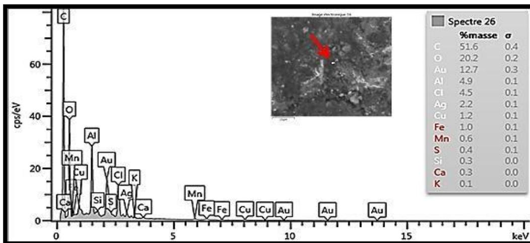
Fig. 15: EDX data and BSE image showing gold with traces of Cu, Fe and Mn.
